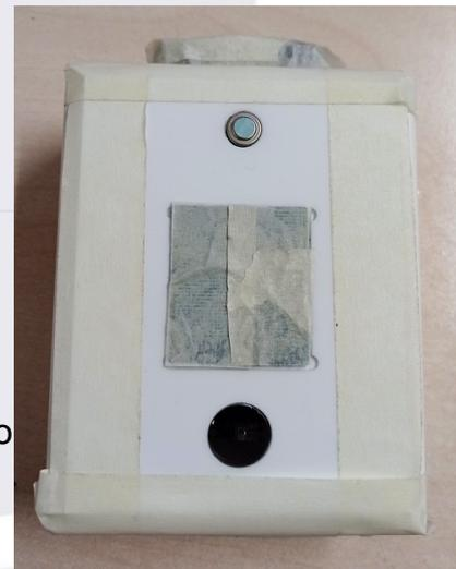
2- Apply a few thin layers all over the device. 2 or 3 layers will be enough. Spray from 20 cm or so, a couple of seconds each pass as you move from one side to the other.
