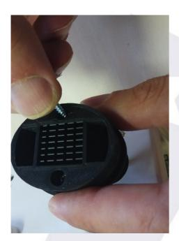
Prepare the sensor: introduce the screws in the two round holes until the tip appears on the back of the cover.
