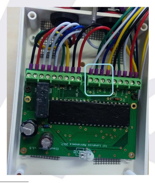
Sometimes, when loosening the screws in the green terminal plugs, the part that holds the cable does not move - so the cable is not freed. In this case, press firmly the screwdriver on the screw, give a sharp (but light!) blow downwards on it until you hear the "click" and unscrew again.
