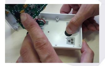
Remove the protective lid from the back putting pressure on it with your finger.
