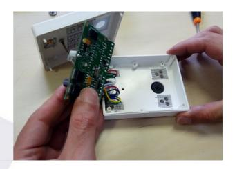
Once the back of the box is separated, insert the sensor cables through the first ventilation hole, as shown in the image.
