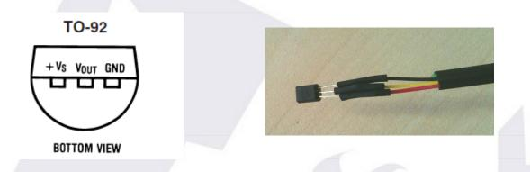
In the example image, +Vs is connected to RED, Vout to YELLOW, GND to BLACK wire.
