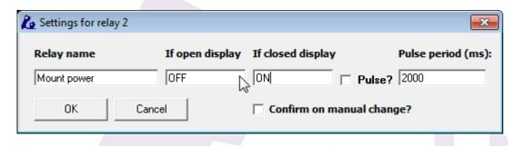
... please continue to do the same for the CCD power and observatory lights – don't forget the lights will be off if the relay is closed!
