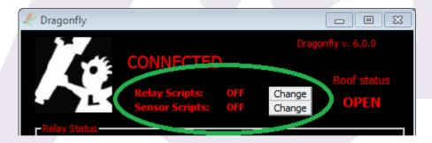
The software can execute a script every time a sensor or relay changes. Check the <u>Automated control – on / off scripts</u> section.
