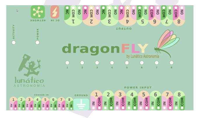
...you'll note we've used this naming convention for labelling the input and output connectors.
