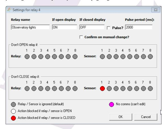
Clicking on each small circle, we can block the relay action (upper row, blocks opening; lower row, blocks closing) on each condition – relay or sensor open or closed.
