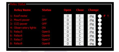
Notice both the "P" and the "!" on the right side, roof relay; the "P" means it is pulsed, the "!" means you'll be asked for confirmation before any action takes place.
