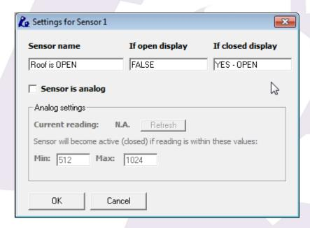
For the roof (roll off roof) we suggest using two switches, one for signalling "open" and another one to signal "closed", this way we will notice should the roof stop mid-travel.
