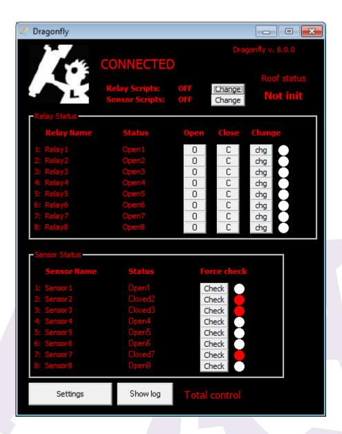
We'll focus, for now, on the two big areas, upper one for relays, lower for sensors. It's easy to see there are 8 rows of relays and 8 of sensors, just as in the physical box.
