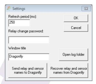
The refresh period establishes how often the sensors (and relays) will all be checked, one at a time. It can have any value between 100 and 60000 ms. For local area networks, 250ms or even faster is okay. If you will be connecting from far away, via internet, using a higher value (1000ms or so) may be better – you can always force the immediate check of a sensor by clicking on that sensor's "Check" button.
