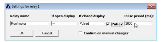
You can name the relay and what should appear when it's closed and open. You can also define it to be a "pulsed" relay, as appropriate in the roof motor configuration. The pulse period, you surely guessed it, is the approximate duration of the pulse in milliseconds.
