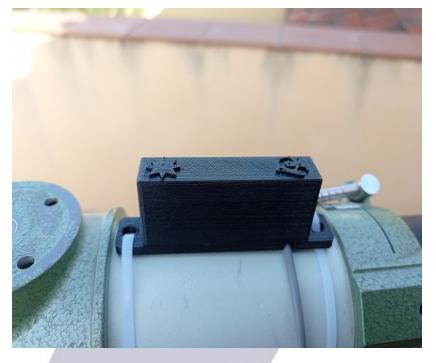
In any case please test, and if needed shim the sensor so the horizontal / parked detection is ensured.
