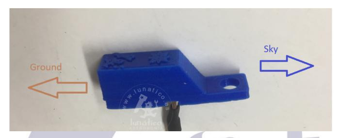
The cable can be bent to both sides of the sensor for easier installation.
